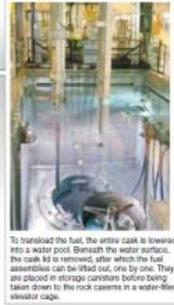
To stabilize the fuel, the entire cask is lowered into a water pool. Beneath the water surface, the cask lid is removed, after which the fuel assemblies can be lifted out, one by one. They are placed in storage canisters before being taken down to the rock caverns in a water-filled elevator cage.
