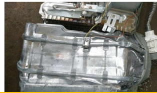
Lead coated boiler
