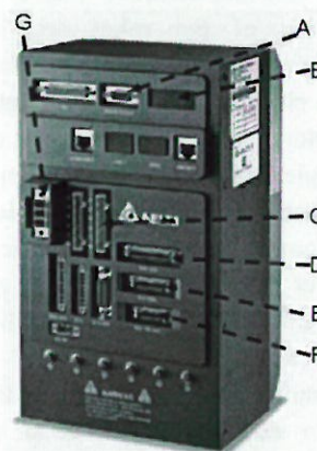
Fig. 3. The PLC-based controller(ASDA-SM)
