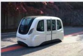
High-Strength Light-Weight Body by CFRP
