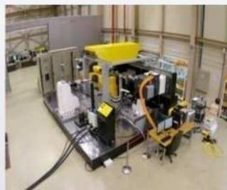
High speed wheel/rail contact simulator
