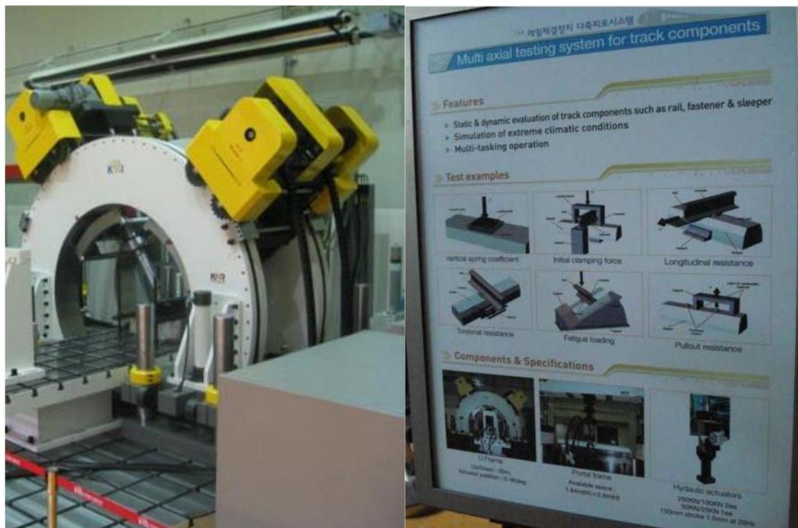
圖 3-1-14 鐵路測試設備－Multi axial testing system for track components
