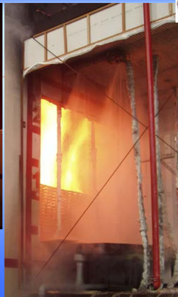
■ Fire propagations with/without water curtain
