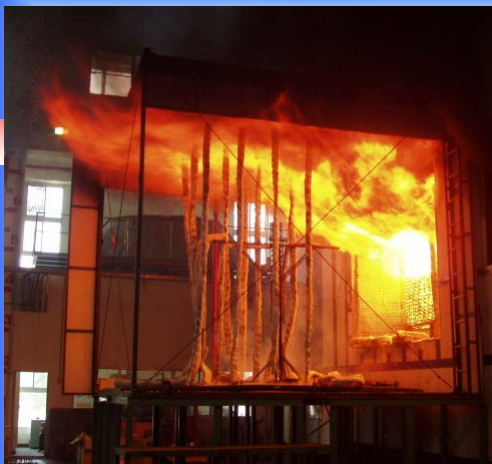
■ Fire propagations with/without water curtain
