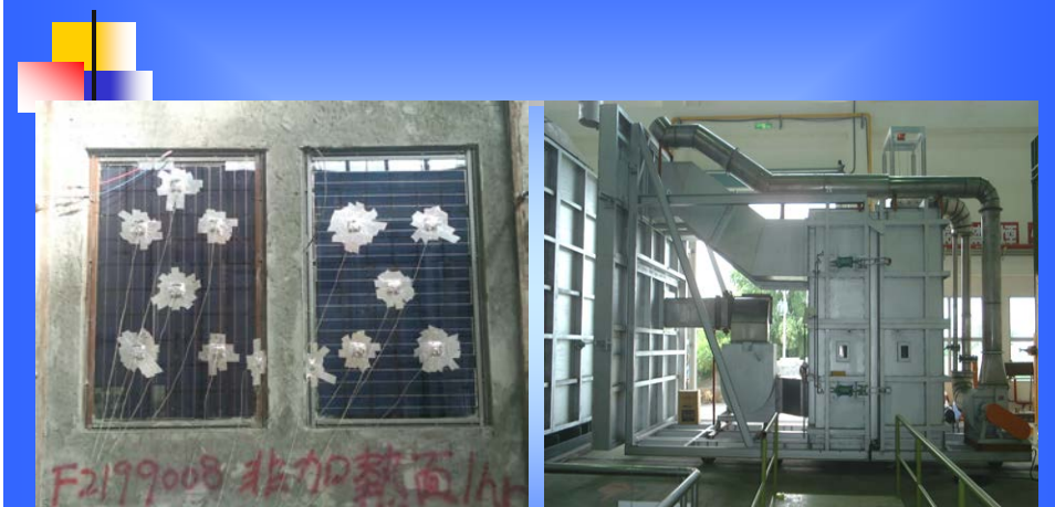
Smoke control performance of fire door
