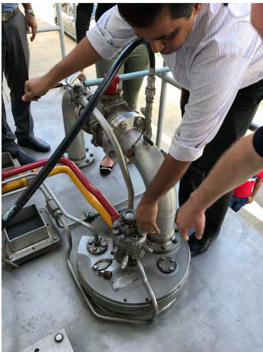
PRATICAL TRAINING: FRAMO CARGO PUMP NORMAL PUMPING & STRIPPING OPERATION (現場 FRAMO 泵浦工廠實際練習壓泵及收艙操作練習)
