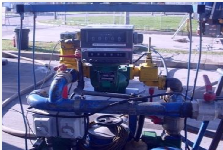
Transfer Pump (ATEX) and Volume Meter (VM) equipped with pulser - (W&M Approved And Sealed)
