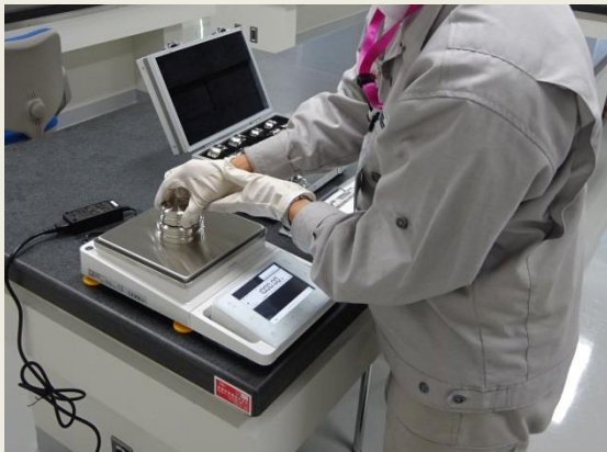
Verification of weighing instruments
