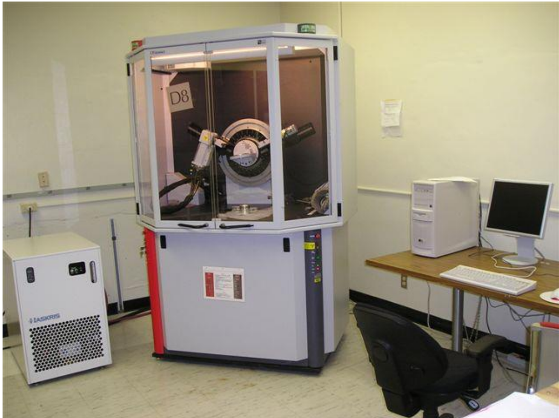
圖 59 XRD分析儀器D8 Advance X-ray diffractometer (Bruker,Germany)
