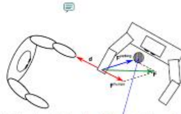
Fig. 3. Schematics of the virtual force F , resulting of the contributions of F^{\text{Human}} and F^{\text{Parking}} . The circle indicates the parking position.
