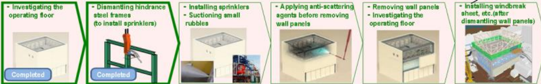
Flow of building cover dismantling
