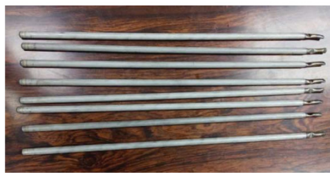
Fig. 1. Photo of homemade SUS316 stainless steel heat pipes.
