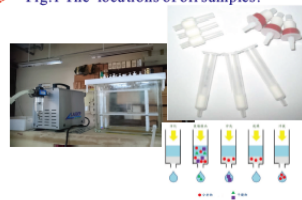
Fig.4 The solid phase extraction (SPE) procedure. The SPE could separate the organic and water phases efficiently, we use this method to separate oil slick from the water.
