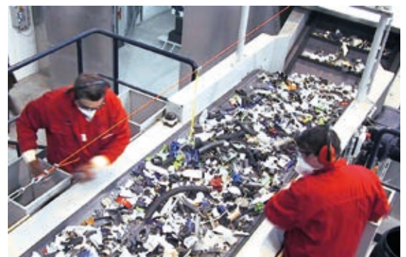
The dismantling and shredding processes used at the dismantling centre in Lünen generate top quality raw materials separated strictly according to type
