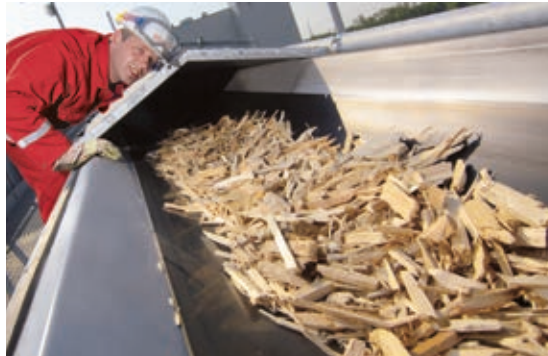
The old wood treated at the timber processing facility is used as a fuel by the neighbouring biomass-fired power plant
