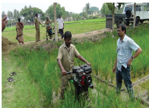
Fig.2 Field view of ride on type paddy weeder
