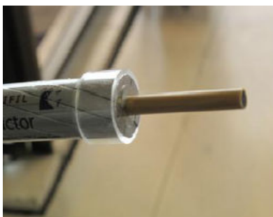
Figure 2: a sample of a conductor with a composite core
