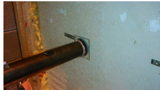
Fig. 2 Impedance tube contacting section of hemp-GGBS wall
