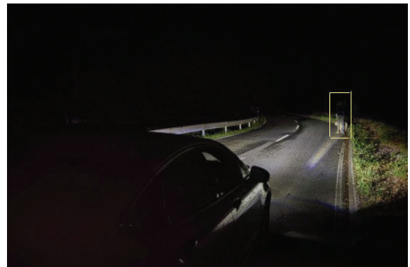
Figure 8: Spot Lighting System
