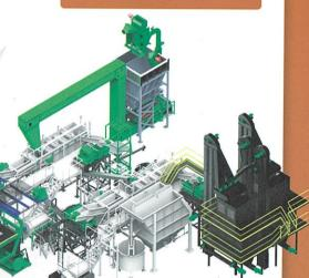
At the PST plant in Tiel, the raw materials present in shredder waste are separated out. The result is 4 different fractions, for which the various machines in the plant have each been painted in their own colour, broadly along the following lines: metals (red), plastics (green), fibres (orange) and minerals (yellow).
