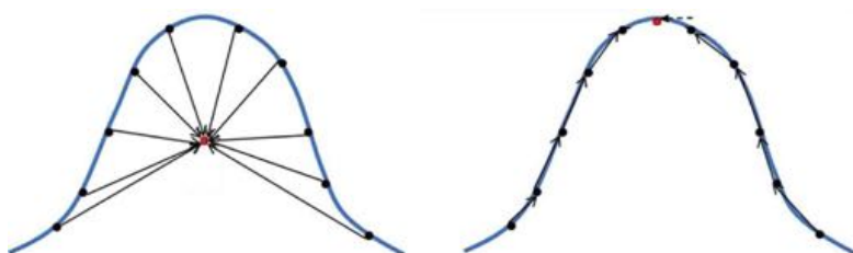
(Left): Arithmetic mean and (Right): Intrinsic mean of data points lying on 1-D manifold.
