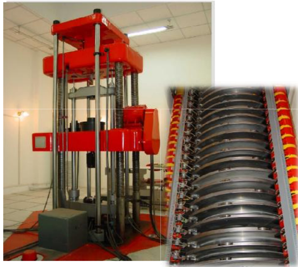
300kN Force Standard machine
