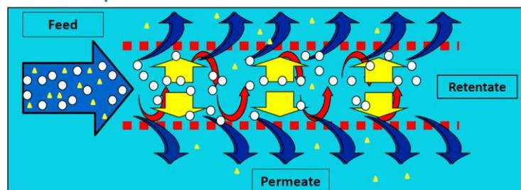
Solutes (proteins, polysaccharides, nucleic acids etc.) larger than the membrane pore size are retained in the retentate while the one with low molecular weight pass into the permeate.
