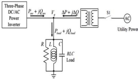
Fig. 1 Test circuit with parallel RLC load
