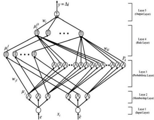
Fig. 3 Network structure of PFNN
