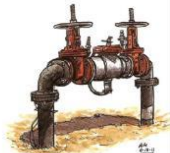
One-way valves to prevent backflow contamination
