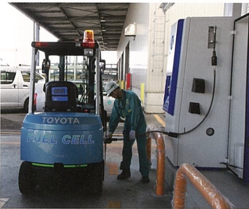
Hydrogen refueling for fuel cell forklifts
