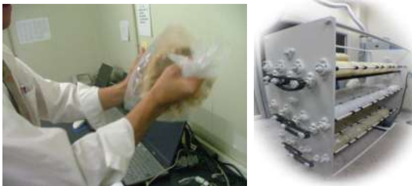
Annex figure 7: An example of mixing procedure; with a plastic bag (left) and with a specialized machine using homogenizing plastic bins (right)
