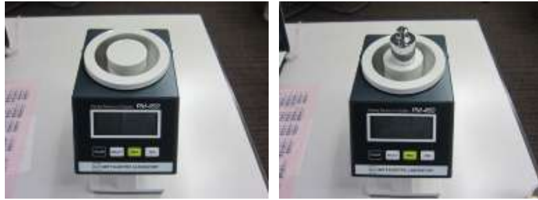
Annex figure 12: Check of the built-in scale
