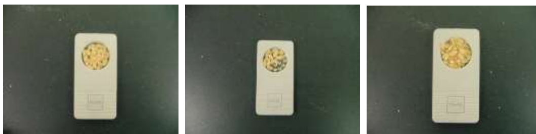
Annex figure 8: Sample set in the tray in one layer. Good (left), too little (middle) and too much (right)
