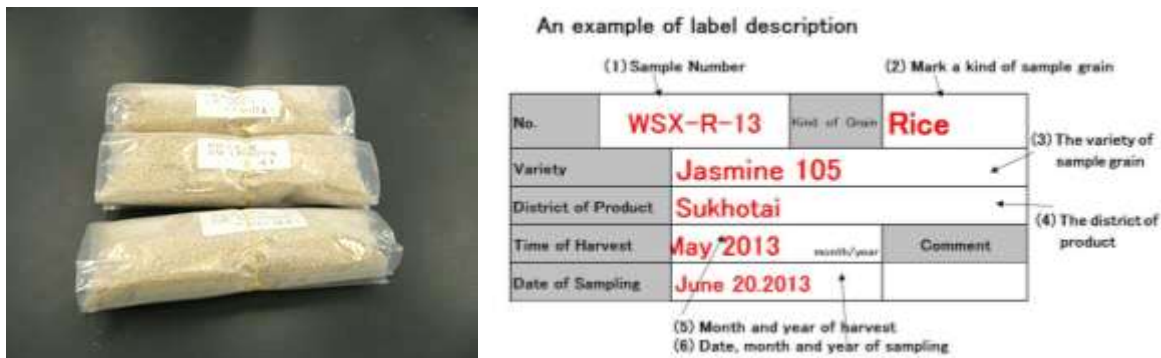
Figure 22: Samples mixed and stored in bags (left) and an example of sample label (right)
