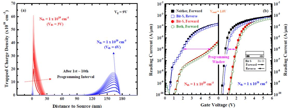
Fig. 2. (a) Iterative results of spatial distributions of trapped charges in light and heavy DS Schottky barrier charge-trapping cells. (b) Programming window of two-bit/cell DS Schottky barrier cells using forward and reverse two-bit/cell reading.
