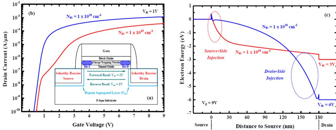
Fig. 1. (a) Schematic structure, and (b) drain current, of a two-bit/cell DS-structured Schottky barrier charge-trapping cell. (c) Channel conduction-band diagrams in light and heavy DS Schottky barrier charge-trapping cells at initial programming.
