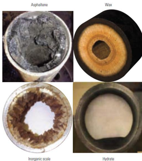
Common deposits that form in tubulars during hydrocarbon production. Wax and hydrate deposition mainly result from a temperature decrease, while asphaltene precipitation may be triggered by changes in pressure, temperature and composition. Inorganic scales arise from changes in pressure, temperature and composition of aqueous fluids that accompany hydrocarbon production. (With kind permission of Springer Science and Business Media.)
