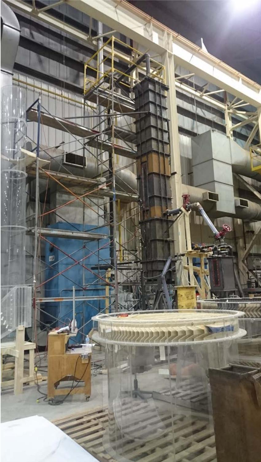
圖 25. Nels fluidized bed test tower - used to evaluate the capability to drain solids from a fluidized bed reactor.
