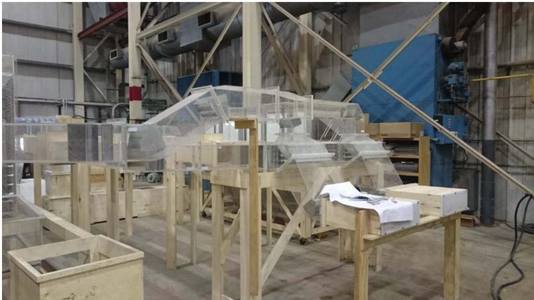
圖 29. ESP installation and ductwork (Multiple ESP unit) used to design the required flow distribution devices within each ESP box to achieve ICAC criteria and design the devices required to achieve the desired flow split between each of the 5 ESP boxes (4 existing and 1 new)
