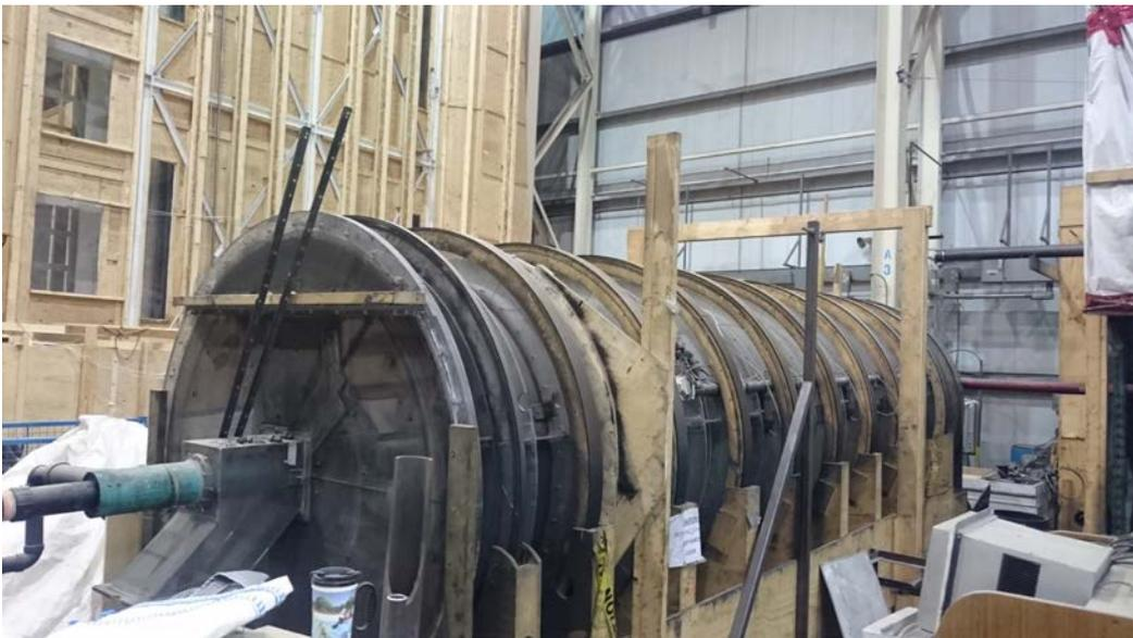
圖 26. Rotational kiln model used to evaluate the current operating characteristics of a nickel carbonyl kiln and developed modifications to increase the production rate of the kiln.
