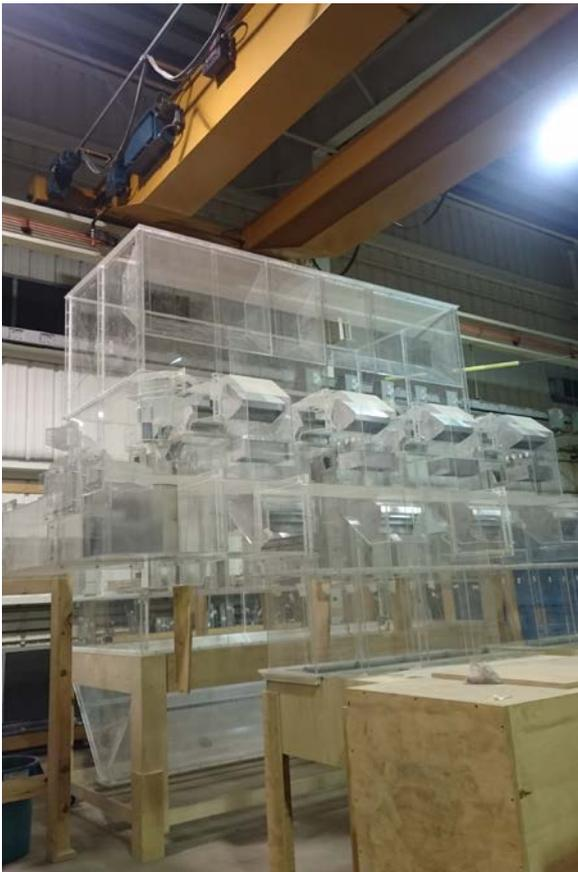
圖 20. Corner fired coal boiler model used to evaluate the current and future design of the OFA system.
