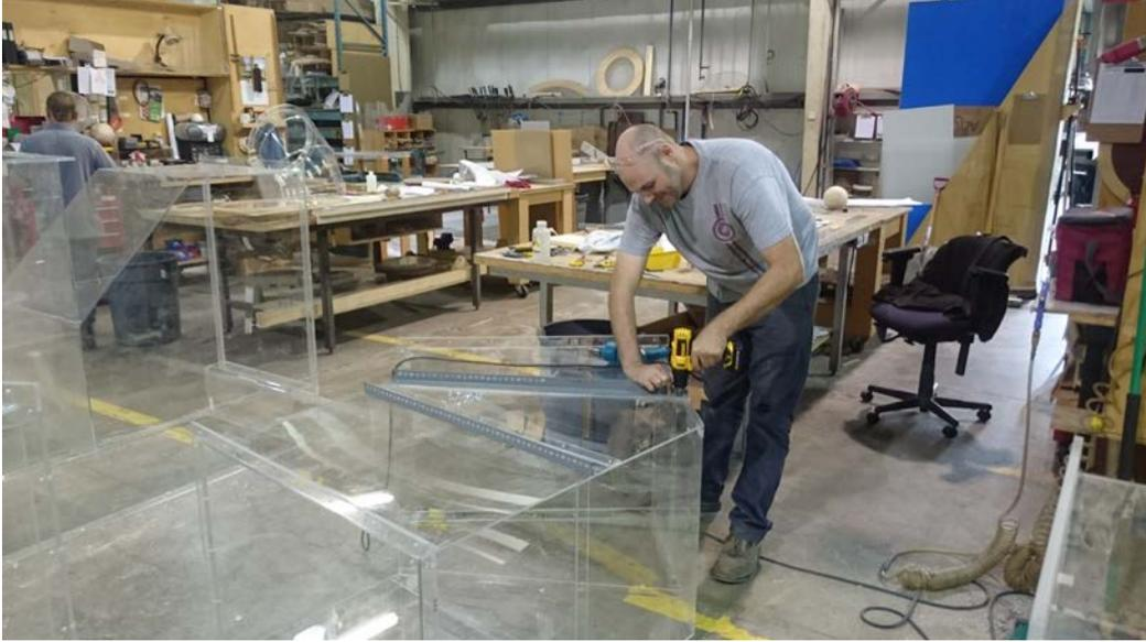
圖 17. Model fabricator making rectangular ductwork for SCR system to ensure satisfactory operation of the full scale unit.
