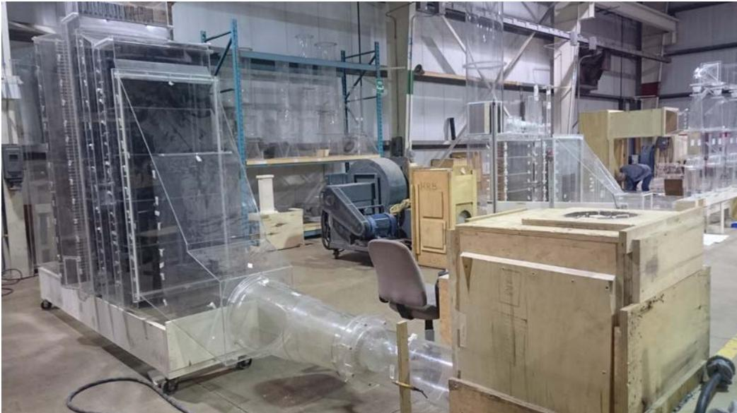
圖 19. Model of HRSG with turbine simulation installed and ID fan (Ready for testing)
