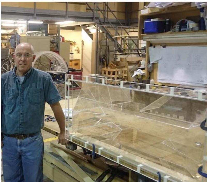
圖 16. Model fabricator making air heater inlet duct for SCR system to ensure satisfactory operation of the full scale unit.
