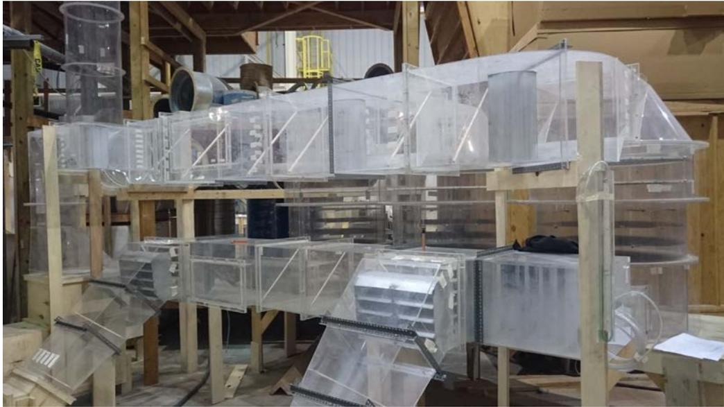
圖 28. Multiple wet scrubber installation model (old unit) , existing unit being modified to remove WFGD bypass system and scrub 100% of the gas flow as opposed to the previous 75-80%. Plant was operating poorly due to changes in the operation of the unit and required modifications to the design to ensure acceptable operation under the revised operating parameters
