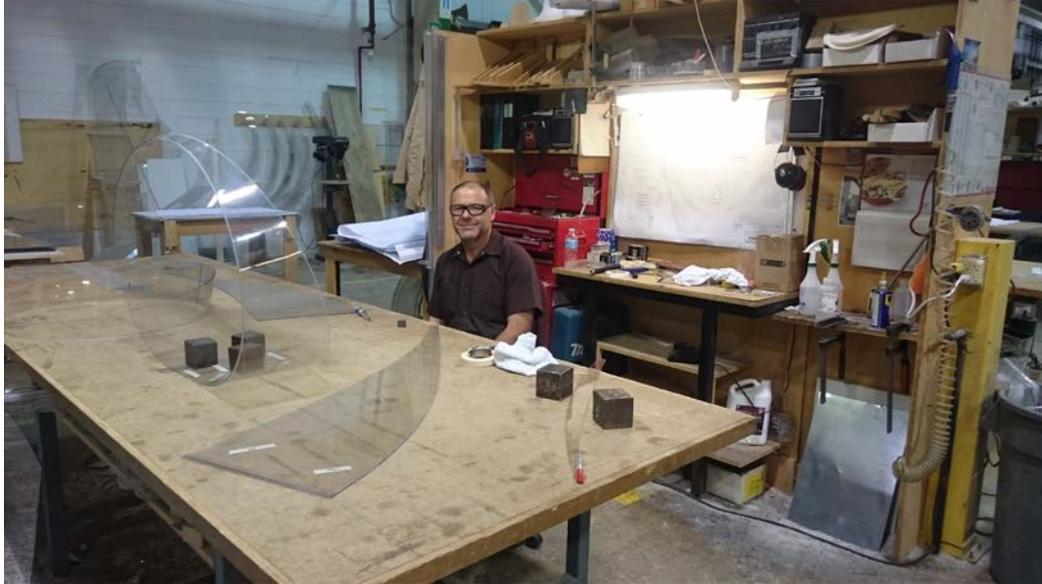
圖 15. Model fabricator making conical transition duct for WFGD to ensure satisfactory operation of the full scale unit.
