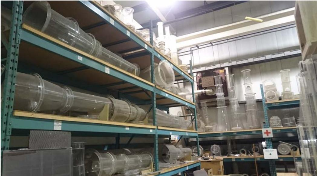
圖 18. Nels inventory of turbine exhaust diffuser models. Used to correctly simulate the flow conditions exiting a gas turbine for the purposes of modeling a HRSG correctly.
