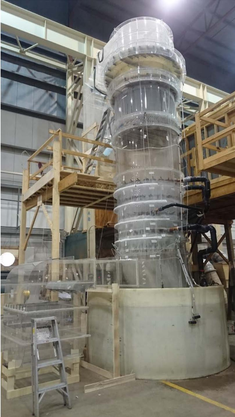
圖 27. Wet scrubber model in operation , tested to ensure satisfactory operation of the full size unit.
