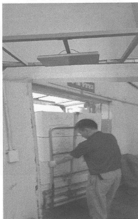
Example of fixed-type RFID reader in the storage room of hospital
