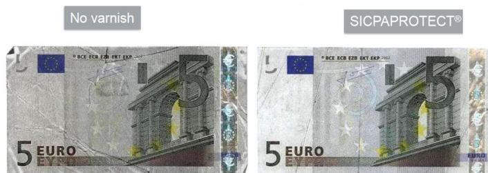
Fritsch test after experimentally ageing the banknotes test on 5 €
