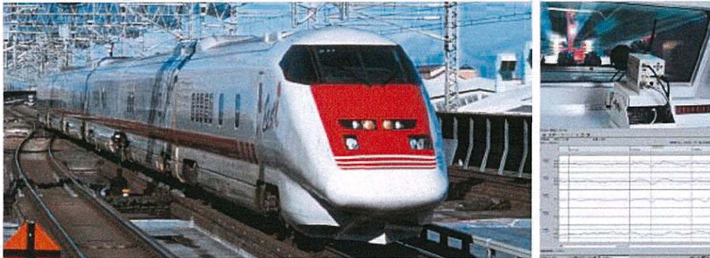
East-i (Shinkansen inspection car for electric equipment and track)
