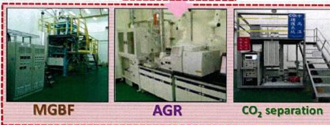
➤ Acid Gas Removal: Stability of desulfurization solid sorbents maintains over 90% during multi-cycle tests.
