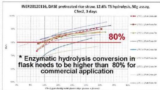
Evaluation of enzymatic hydrolysis of the pretreated rice straw by Novozymes
