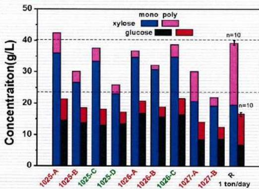
Rice straw hydrolysate obtained after pretreatment system of the pilot plant
