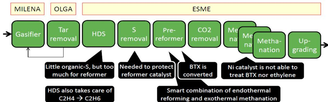
Gasifier: Fluidized Bed Gasifier operating at  $\sim 800^{\circ}\text{C}$
