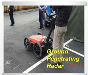
Detect underground pipelines
