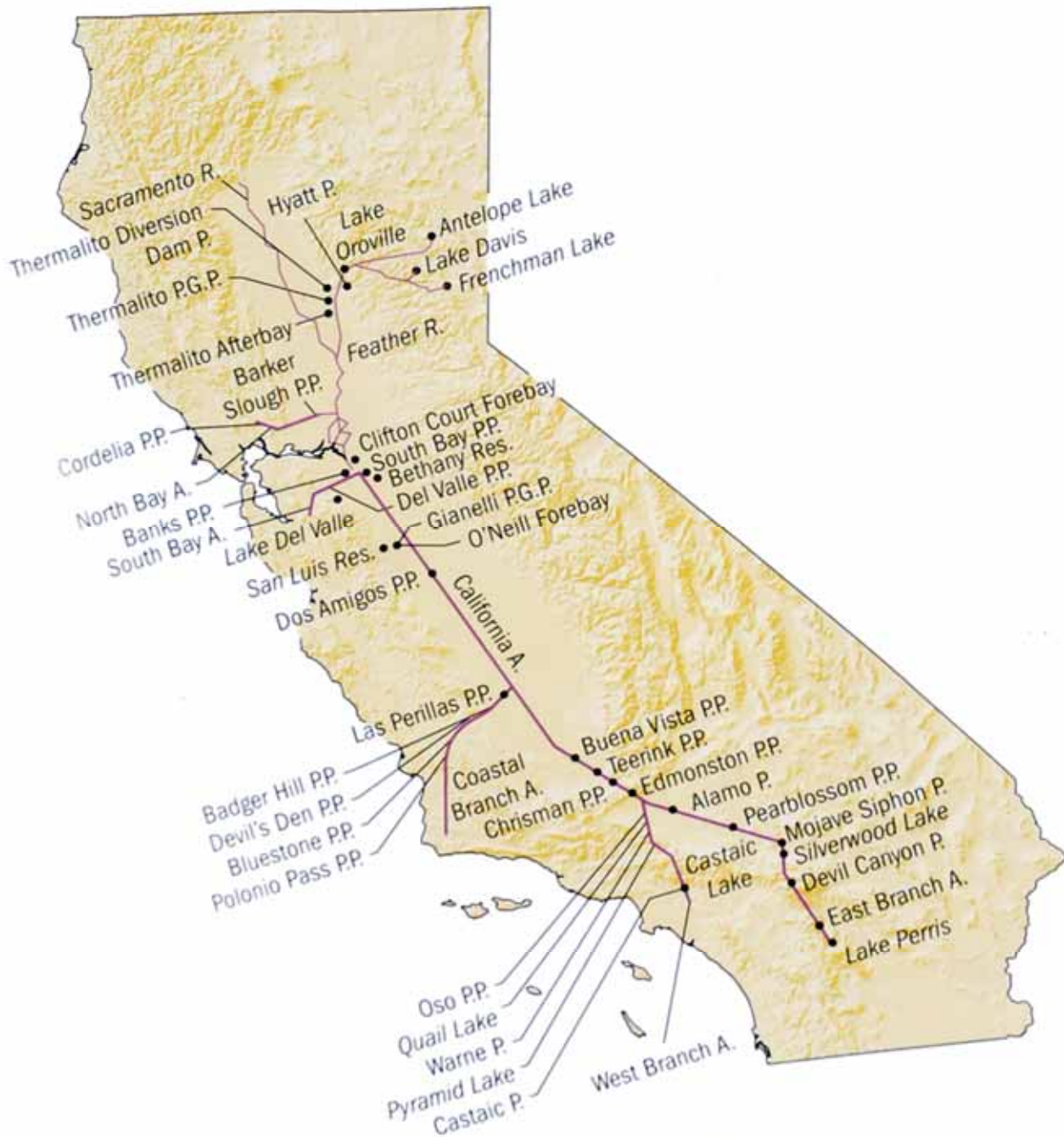
Map 13. State Water Project facilities. (Picked up from two maps in California Department of Water Resources 1998.)
