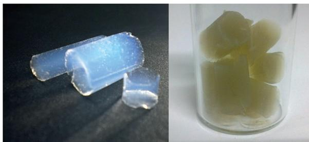
Fig. 6 Silica aerogel before (left) and after (right) catalyst impregnation.
