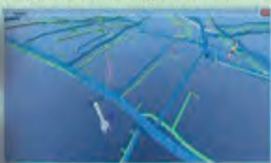
Vector theme (pipelines) used to select voxels in a voxel model. Diameter and material type has been used (attributes in table from shape file).
