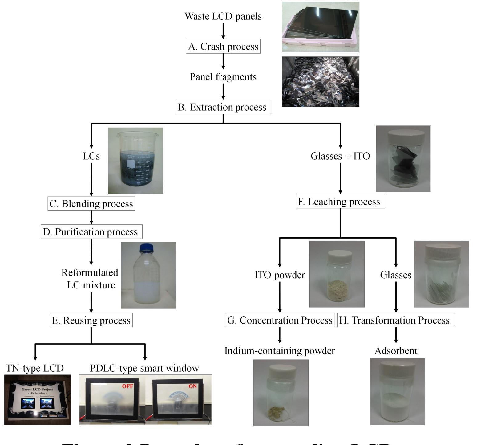
Figure 2 Procedure for recycling LCD
