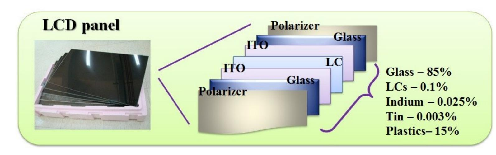
Figure 1 The brief structure of a LCD panel
