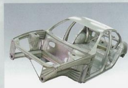
White automobile body using HITEN (high-strength steel sheet)
