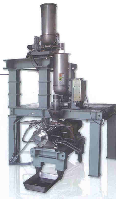
実験機：粉体定量供給機+KRCニーダ Test machine: Improved loss-in-weight feeder + KRC kneader
