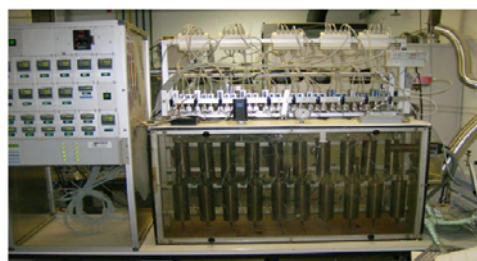
10 Tube screening test unit
