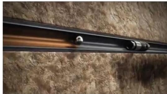
Step4.放置高強度液裂球(High-strength frac balls)
