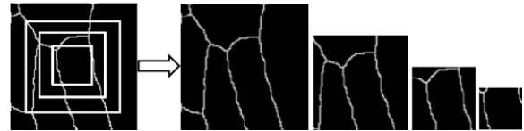
Figure 2. Inward partitioning of thinned image resulting in four sub-images of various dimensions ( 128 \times 128 , 96 \times 96 , 64 \times 64 , and 32 \times 32 pixels)
