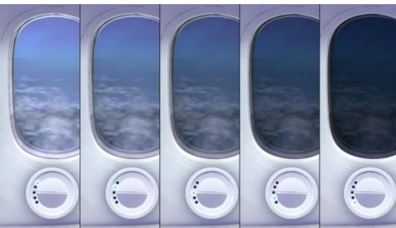
The first electrochromic window in the world (seats on Boeing 787 Dreamliner)
