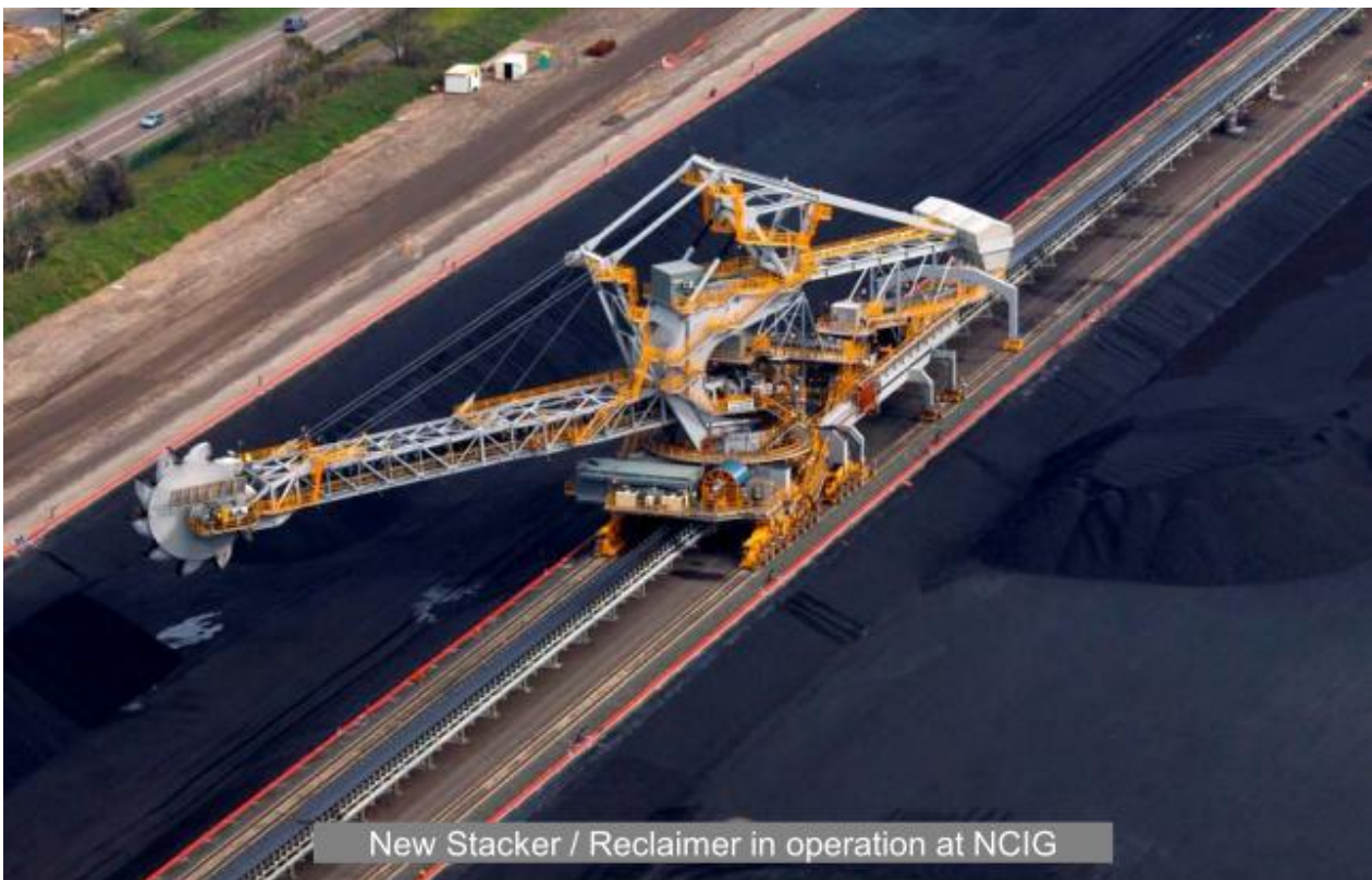
圖167 NCIG 斗輪式堆/取煤機(Bucket Wheel Stacker/Reclaimer)
