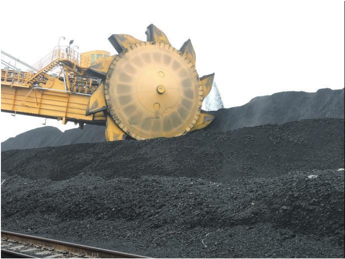
圖154 PWCS 斗輪式堆/取煤機(Bucket Wheel Stacker/Reclaimer)取煤作業
