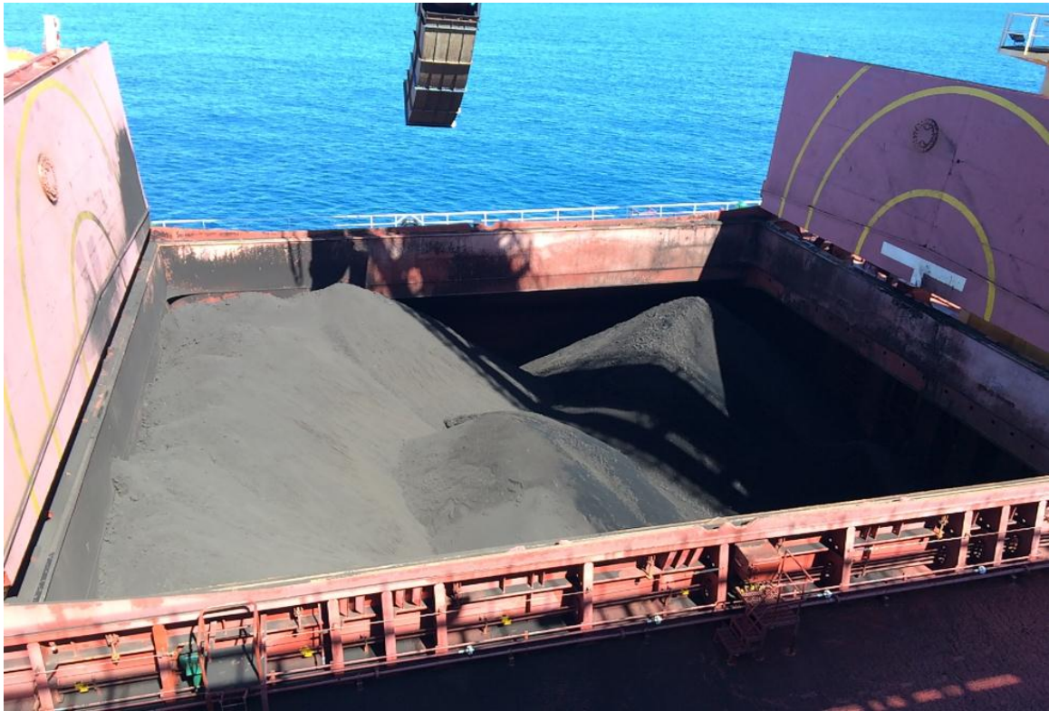
圖49 Kalimantan Floating Terminal裝煤至煤輪
