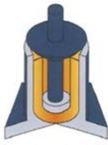
Piercing of a centre hole with a mandrel
