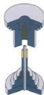
Insertion of mandrel into blocker
