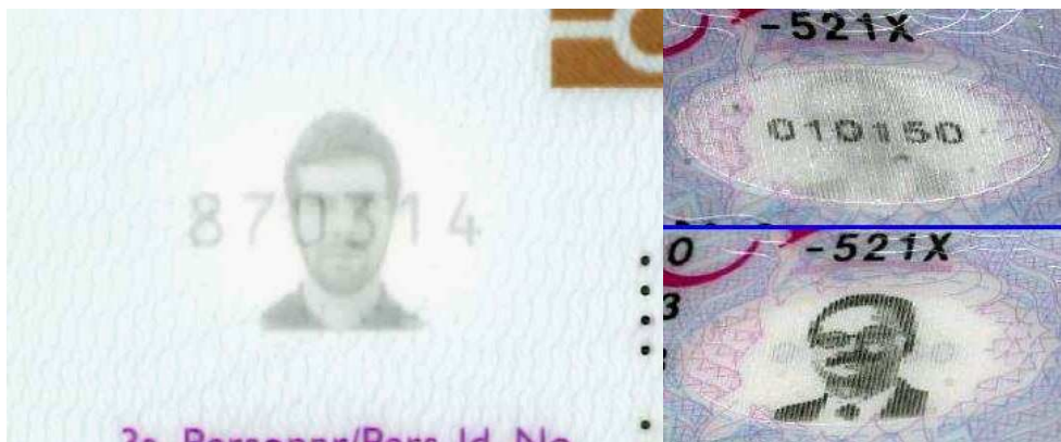
圖3.9 CLI/MLI (changeable/multiple laser image)
