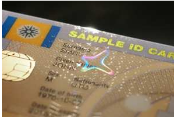
圖3.8 光學可變表面(Sealys Optically Variable Surface)
