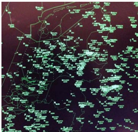
ht Information without height filters. Radar screen of Amsterdam Flight information without height filters.
