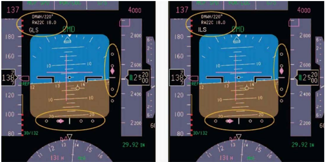
A pilot barely finds any difference between an ILS and GBAS approaches
