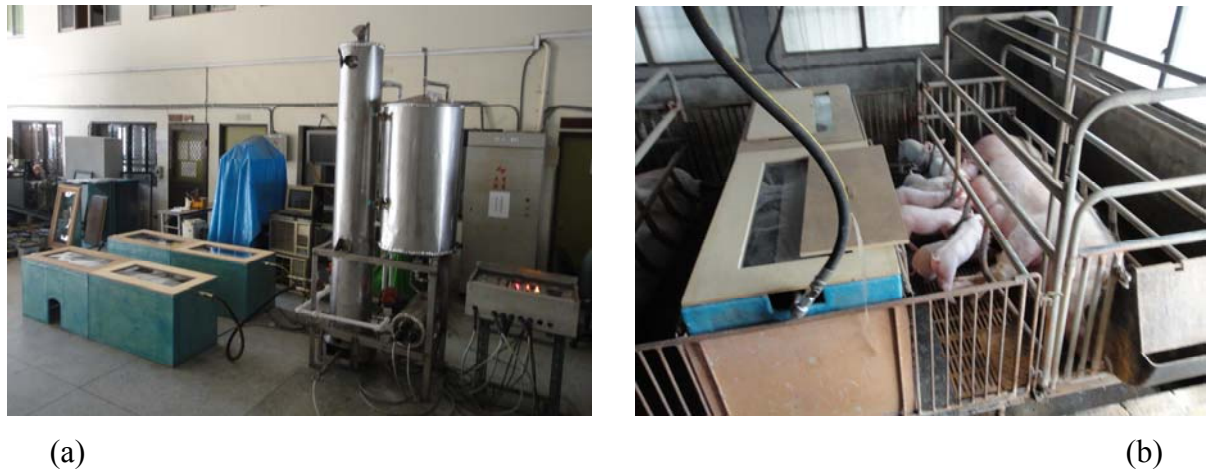
Figure 2. (a) The simulation test of the water heating system. (b) The field test in the farrowing house of the little pig farm.
