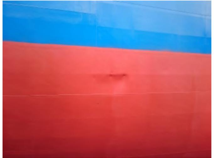
**The ship's starboard side hull has white point and little structure damage.**
