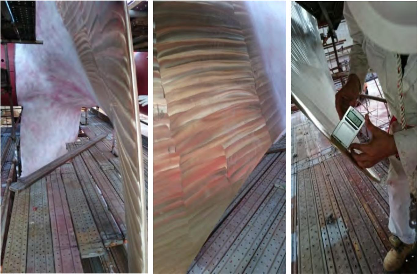
**Inspection of propeller, make sure the surface quality and confirm the propeller blade thickness.**
