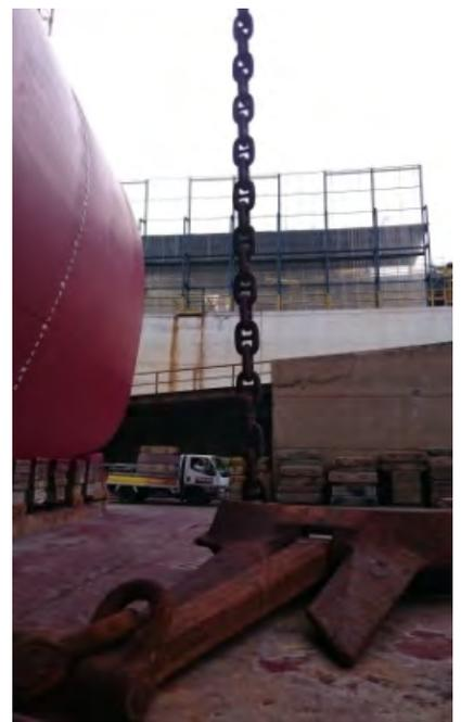
Inspection for anchor & chain (P&S) then, calculate chain's numbers and painting.
