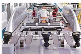
▼ 弓網檢測系統 Pantograph-Catenary Inspection System
