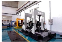
▲ 測力輪對標定試驗台 The Instrumented Wheelset Calibration Test-bed
