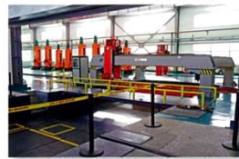
▲ 轉向架更換設備 Bogie Replacement Equipment
