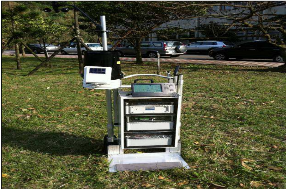
Mobile Radiation/Weather Monitoring Cart
