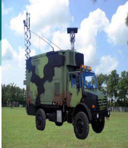
A vehicle supported by the special forces carries the MERM to execute the patrol detection on the road.
